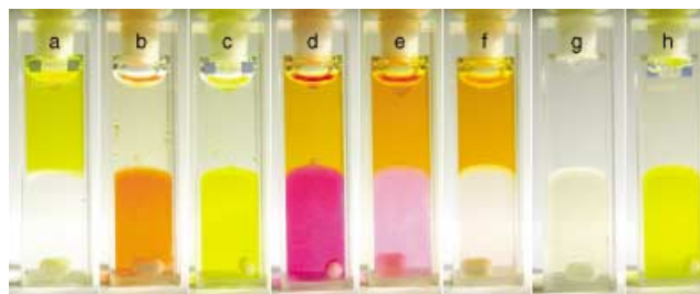
Figure 2. a) 1- n -Butyl-3-methylimidazolium hexafluorophosphate, [\text{bmim}][\text{PF}_6] (lower phase), 4',7-dihydroxyflavylium perchlorate in 0.01 M HCl, \text{AH}^+ species (upper phase); b) after moderate shaking, \text{A} species (lower phase); c) after vigorous shaking, \text{AH}^+ species (lower phase); d) after making the aqueous phase alkaline (pH 12) with minimum shaking, \text{A}^- (lower phase), \text{Ct}^{2-} (upper phase); e) after moderate shaking; f) after vigorous shaking, \text{Ct}^{2-} species (upper phase); g) after reacidification of the aqueous phase and vigorous shaking, \text{Ct} species (lower phase); h) after irradiation of the ionic-liquid phase at 366 nm, \text{AH}^+ species.
